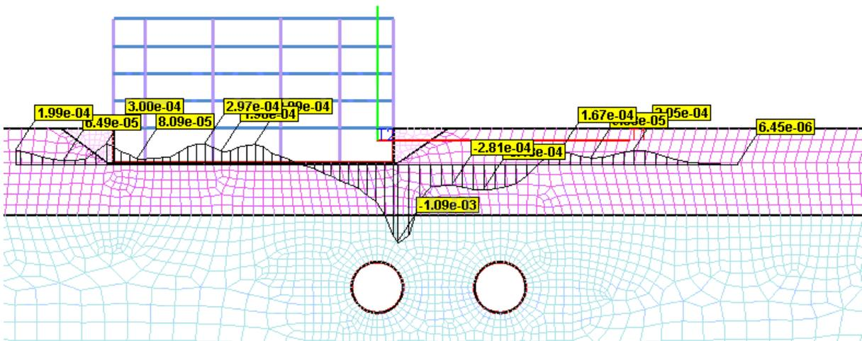
**Figure B1.22** Predicted horizontal strain distribution profile based on FEM analysis under non-greenfield conditions for assumed  $V_{L,95\%}$  - both tunnels.
