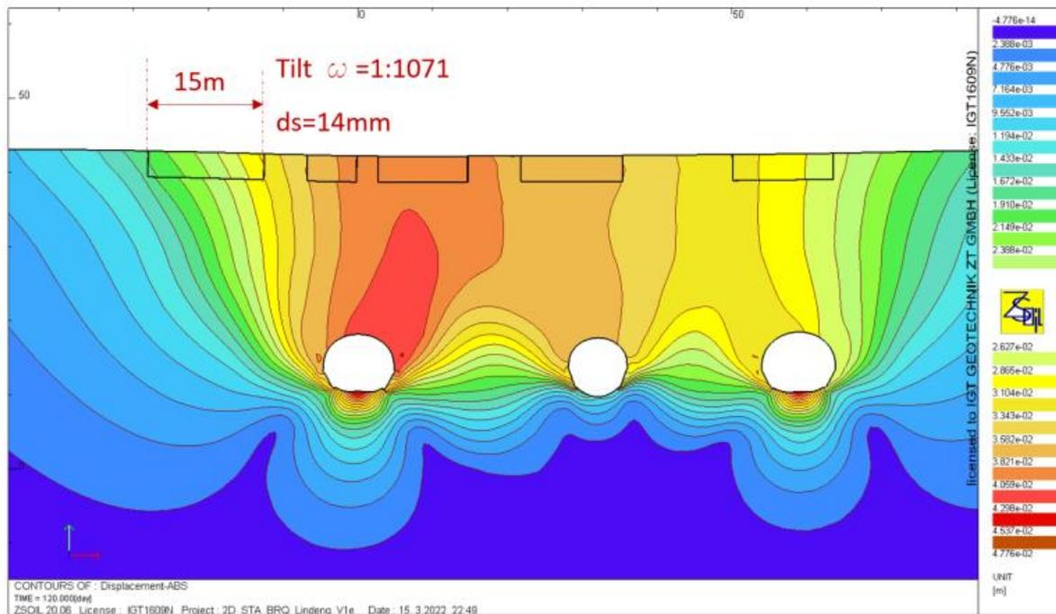
**Figure B1.11** Vertical displacement with maximum tilt of buildings above the tunnel
