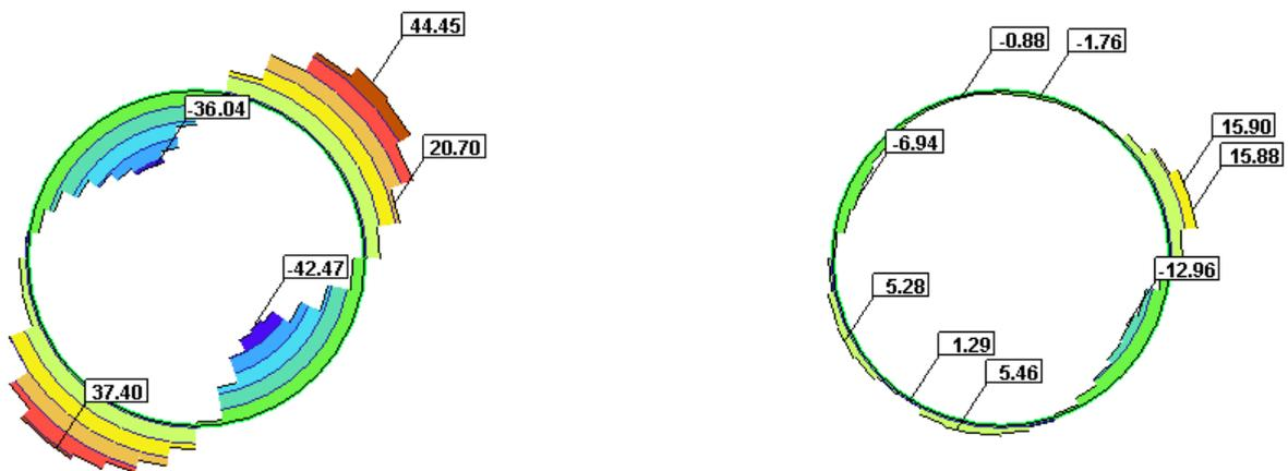
**Figure B1.8** Shear force  $Q$  [kN/m] at  $V_{L,95\%} = 1.20\%$  for both tunnels.
