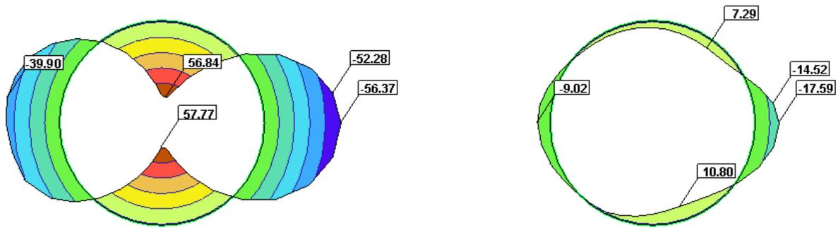
**Figure B1.6** Bending moments  $M$  [kNm/m] at  $V_{L,95\%} = 1.20\%$  for both tunnels.
