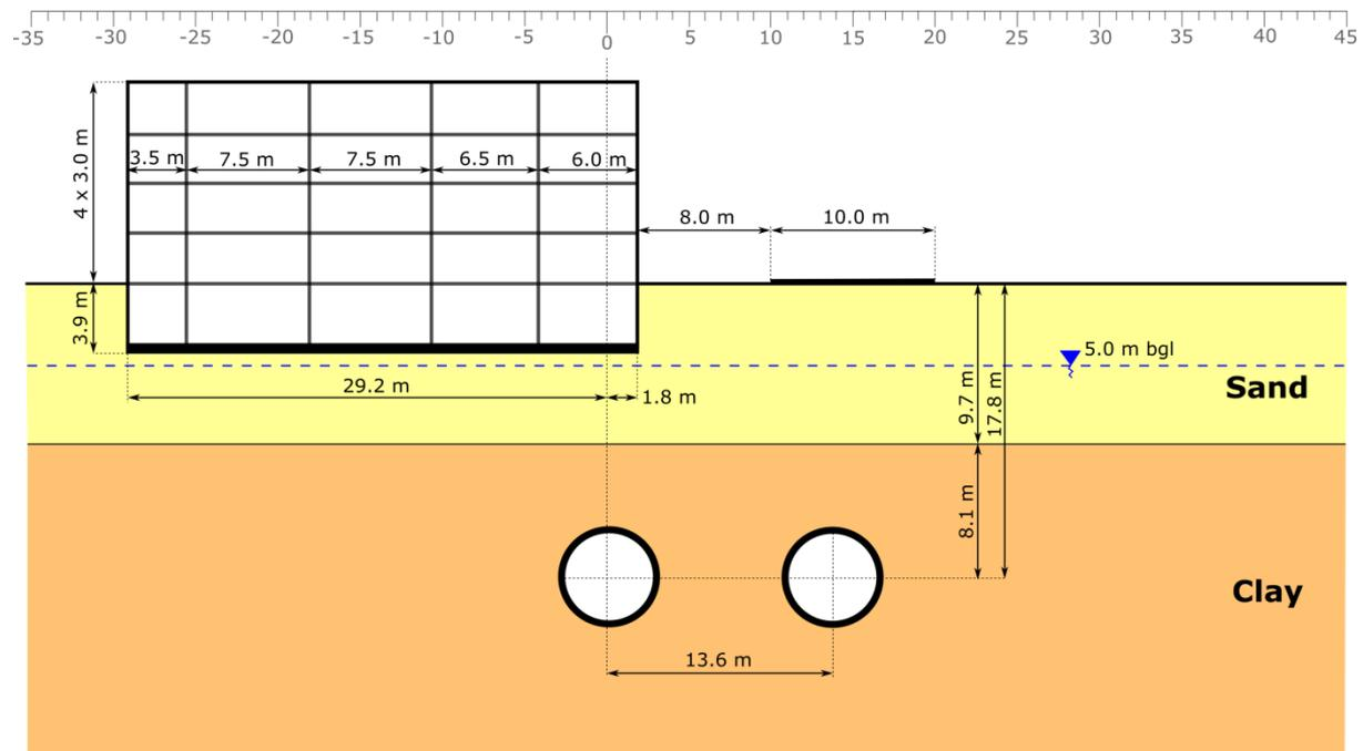
**Figure B1.1** Geometry of the considered design example.
