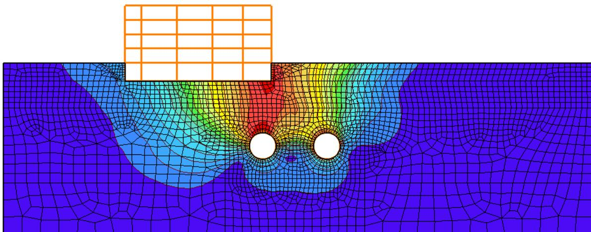
**Figure B1.2** Ground displacement map (extent of the zone of influence) for  $V_{L,50\%} = 0.50\%$ .
