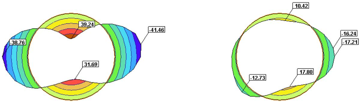
**Figure B1.3** Bending moments  $M$  [kNm/m] at  $V_{L,50\%} = 0.50\%$  for both tunnels.
