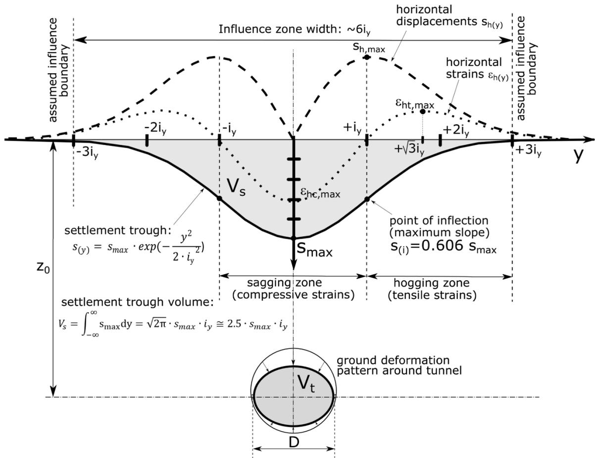
**Figure B1.11** Semi-empirical approach for estimating tunnelling-induced ground deformations (based on model by [17], figure after [6]).
