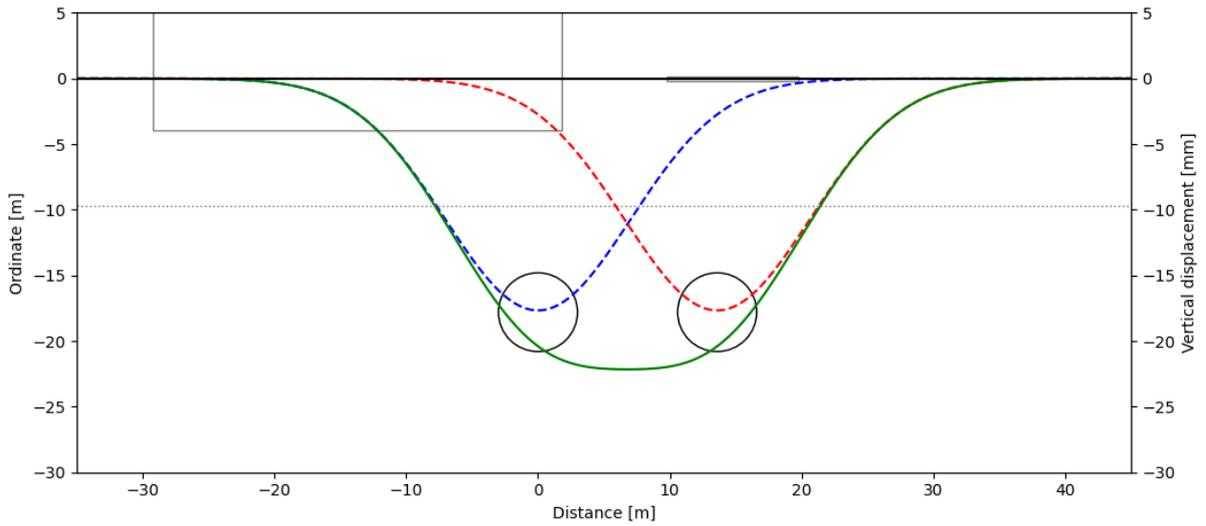
**Figure B1.13** Predicted ground settlement profile based on semi-empirical approach under greenfield conditions for  $V_{L,95\%}$ .
