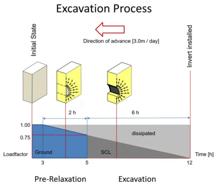
**Figure B2.5** Pre-relaxation function to simulate development of deformation in a 2D-Model
