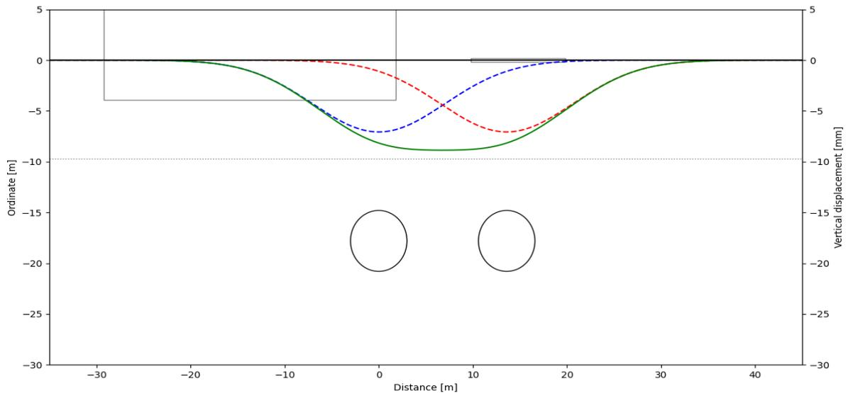
**Figure B1.12** Predicted ground settlement profile based on semi-empirical approach under greenfield conditions for  $V_{L,50\%}$ .
