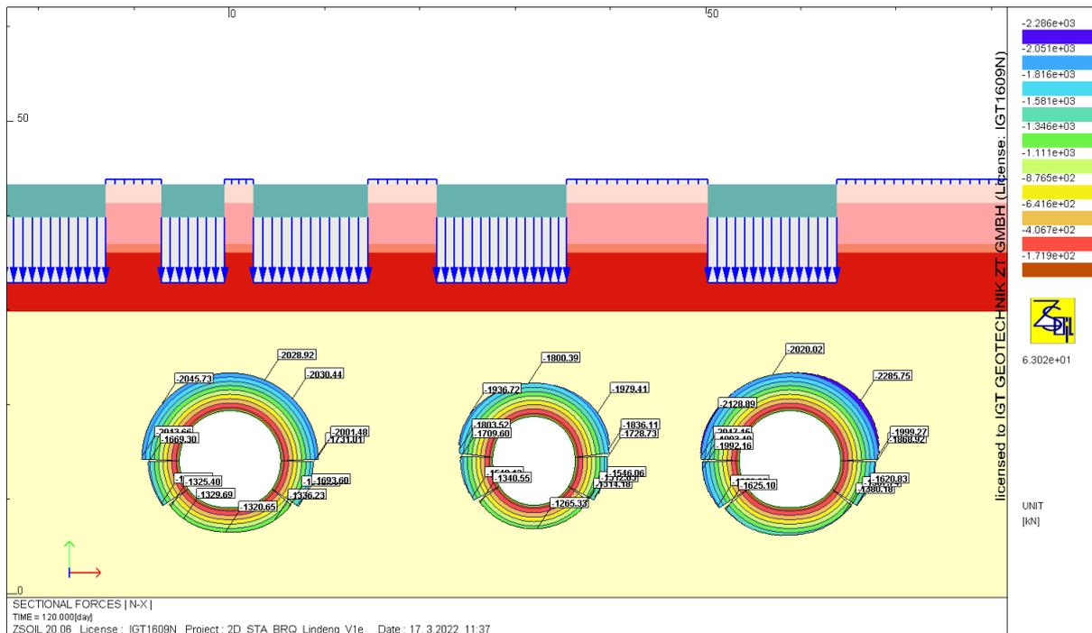
Figure B2.6 Axial Force [kN/m] in the primary lining at end of construction.
