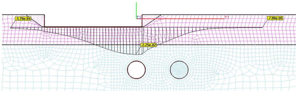
**Figure B1.19** Predicted ground settlement profile based on FEM analysis under non-greenfield conditions for assumed  $V_{L,95\%}$  - first tunnel.
