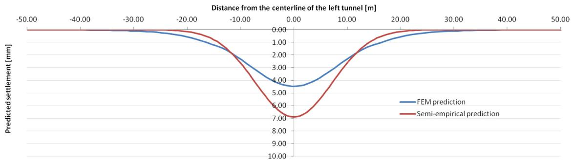
**Figure B1.16** Comparison of ground settlement profiles obtained based on semi-empirical approach and FEM analysis under greenfield conditions for  $V_{L,50\%}$ .
