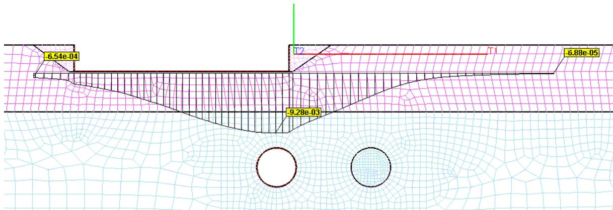
**Figure B1.17** Predicted ground settlement profile based on FEM analysis under non-greenfield conditions for assumed  $V_{L,50\%}$  - first tunnel.
