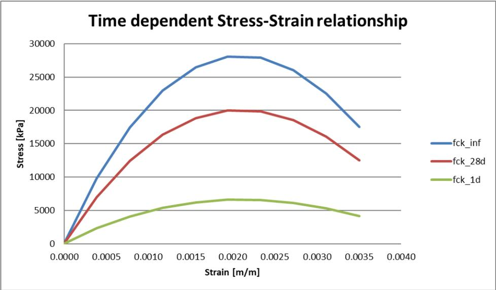
**Figure B2.3** Development of stress-strain curve with time.
