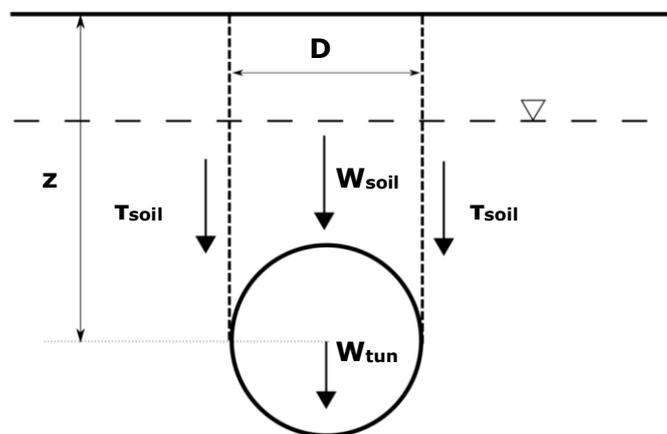
**Figure B1.10** Schematic for uplift limit state verification of a tunnel (based on [16]).
