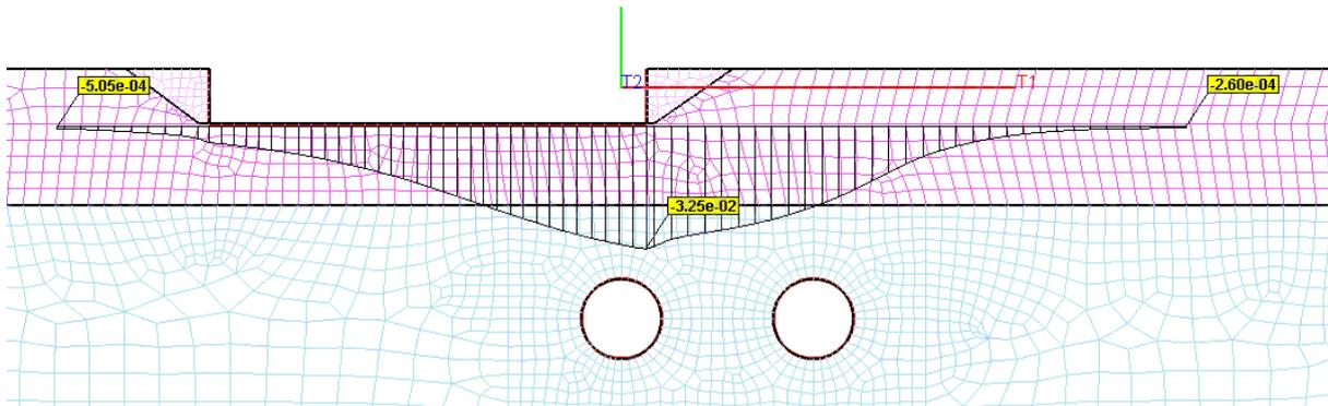
**Figure B1.20** Predicted ground settlement profile based on FEM analysis under non-greenfield conditions for assumed  $V_{L,95\%}$  - both tunnels.
