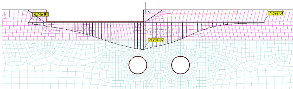
**Figure B1.18** Predicted ground settlement profile based on FEM analysis under non-greenfield conditions for assumed  $V_{L,50\%}$  - both tunnels.
