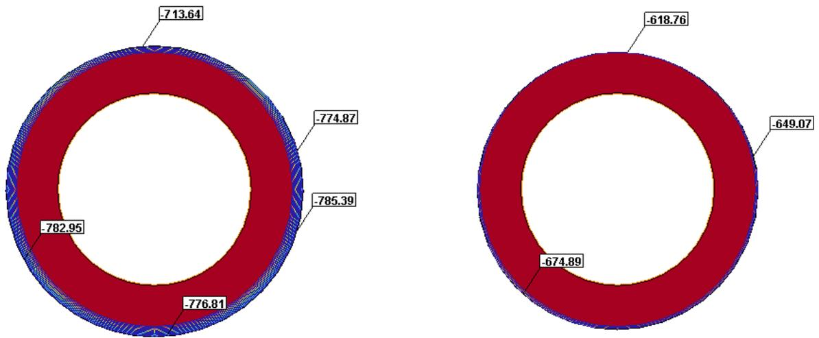
**Figure B1.4** Normal force  $N$  [kN/m] at  $V_{L,50\%} = 0.50\%$  for both tunnels.
