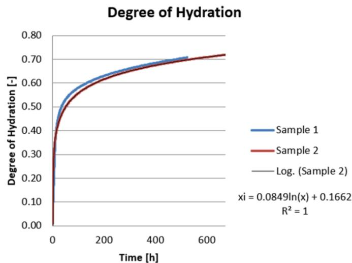
**Figure B2.2** Development of hydration degree with time.
