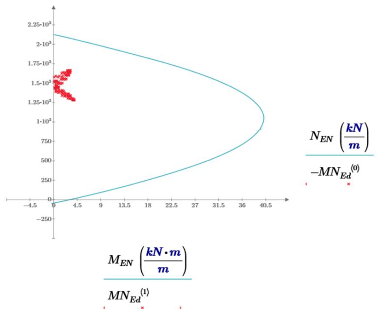
**Figure B1.9** M-N Envelope for the fibre reinforced concrete lining in the pilot tunnel
