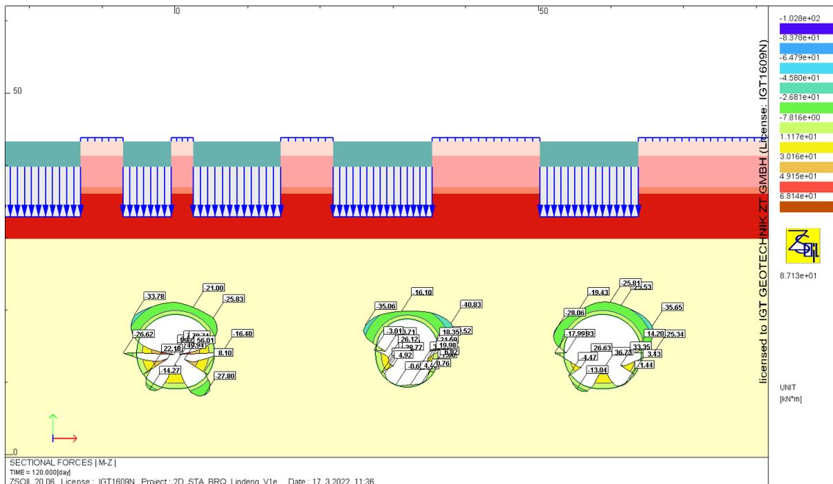
Figure B2.7 Moments [kNm/m] in the primary lining at end of construction.
