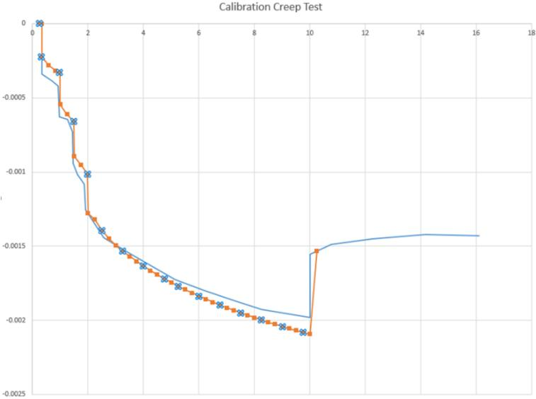
**Figure B2.4** Calibration of creep parameters using a laboratory test.
