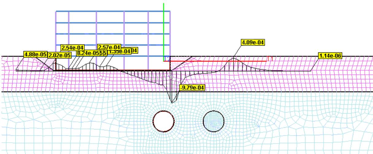
**Figure B1.21** Predicted horizontal strain distribution profile based on FEM analysis under non-greenfield conditions for assumed  $V_{L,95\%}$  - first tunnels.
