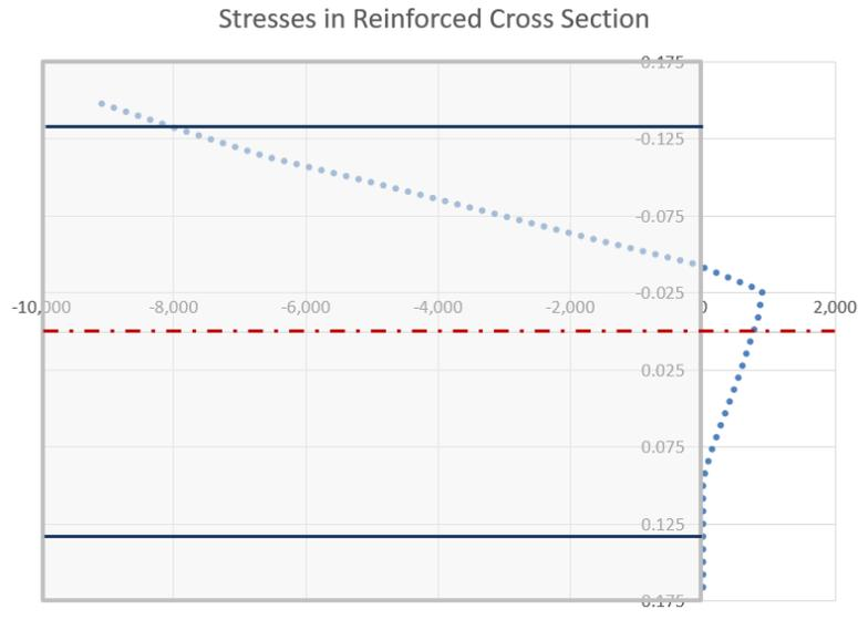
**Figure B1.8** Stress distribution in a typical design section of the primary lining (d=0.35m).
