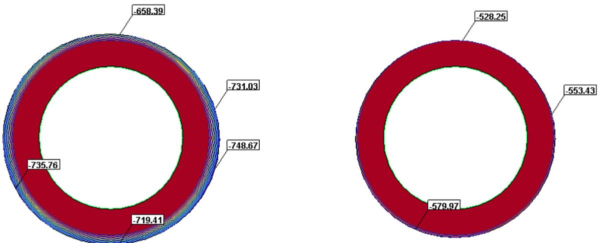
**Figure B1.7** Normal force  $N$  [kN/m] at  $V_{L,95\%} = 1.20\%$  for both tunnels.
