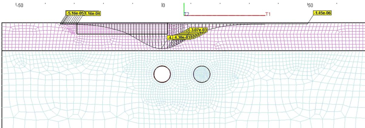
**Figure B1.14** Predicted ground settlement profile based on FEM analysis under greenfield conditions for assumed  $V_{L,50\%}$  - first tunnel.
