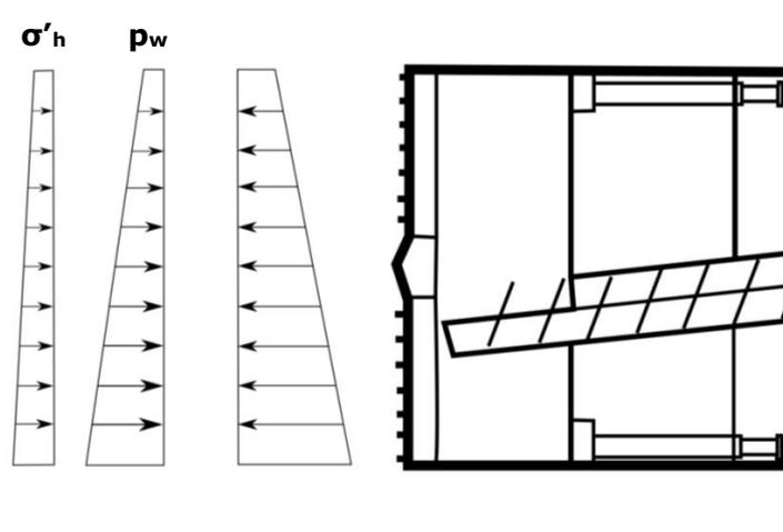
Figure B1.9 Pressures considered in Earth Pressure Balance TBM.
