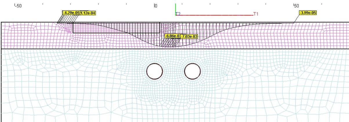
**Figure B1.15** Predicted ground settlement profile based on FEM analysis under greenfield conditions for assumed  $V_{L,50\%}$  - twin tunnels.
