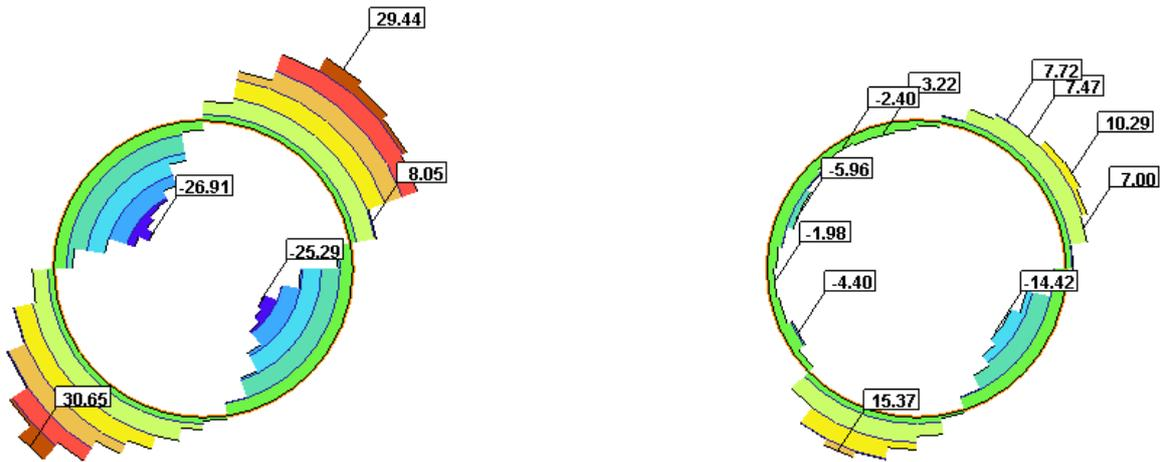
**Figure B1.5** Shear force  $Q$  [kN/m] at  $V_{L,50\%} = 0.50\%$  for both tunnels.
